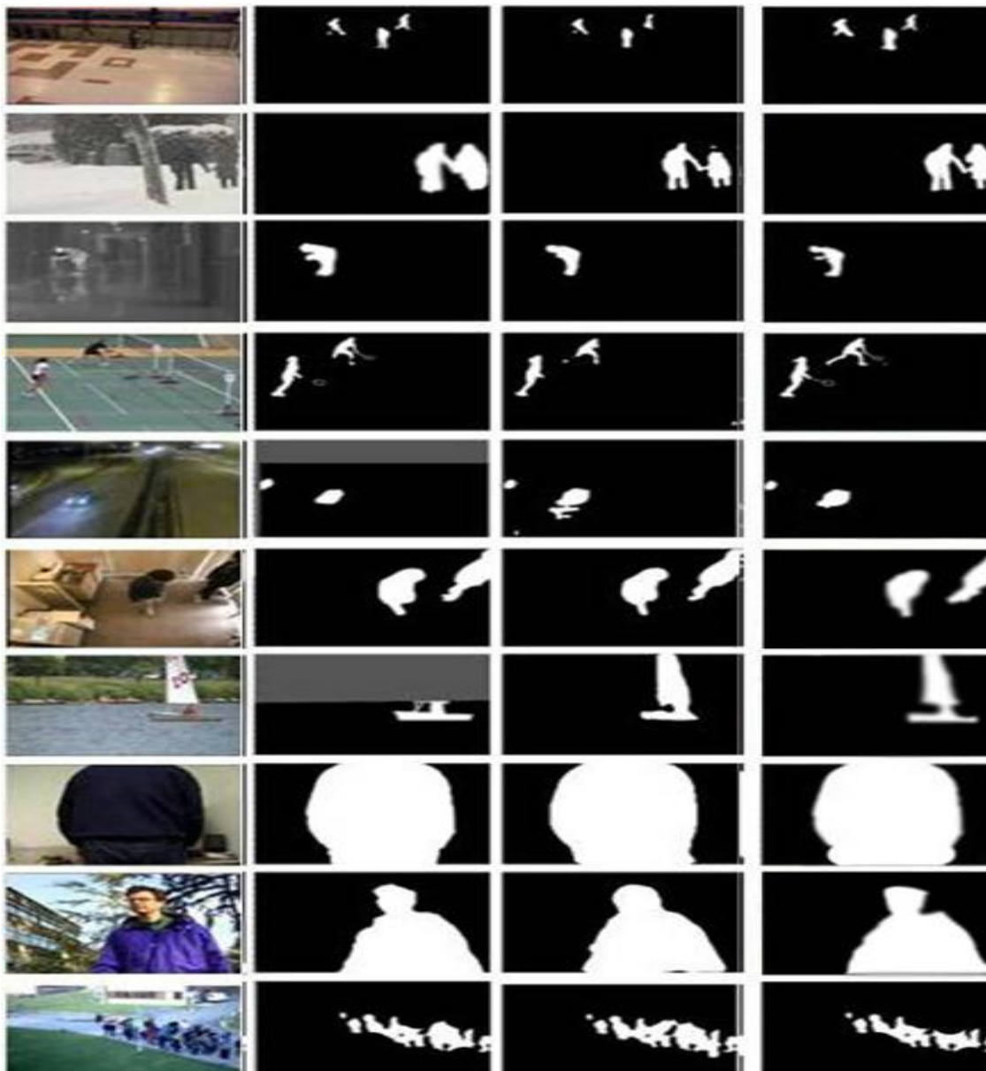
Fig. 6: Comparison of the segmentation outputs: (a) the input images (b) Ground truth images (c) outputs of the CNN (d) outputs of RCNN
