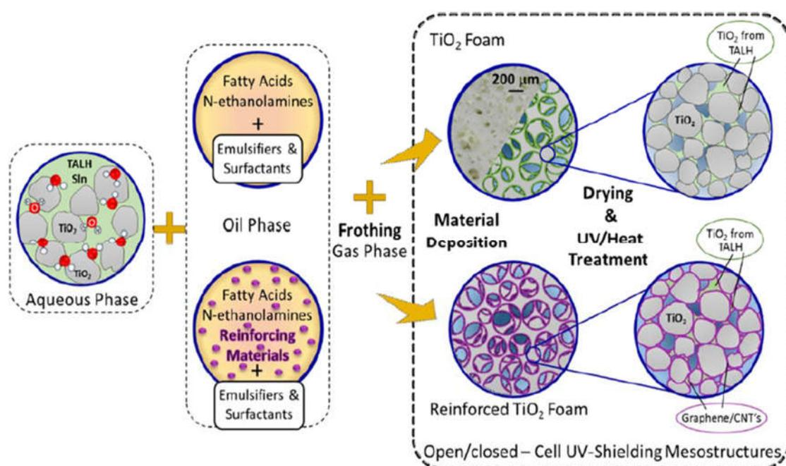
**Figure 2:** Diagram illustrating the preparation process of  $\text{TiO}_2$ : TALH Reinforced and baseline UV-shielding foams. [1-70]
