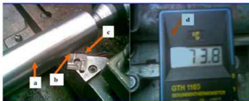
Fig. 3. Temperature measuring device. (a) workpiece, (b): plate, (c): thermocouples and (d): measuring device.
