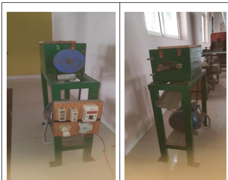
Figure 1: Sectional Views of Single-Shaft Shredder Machine
