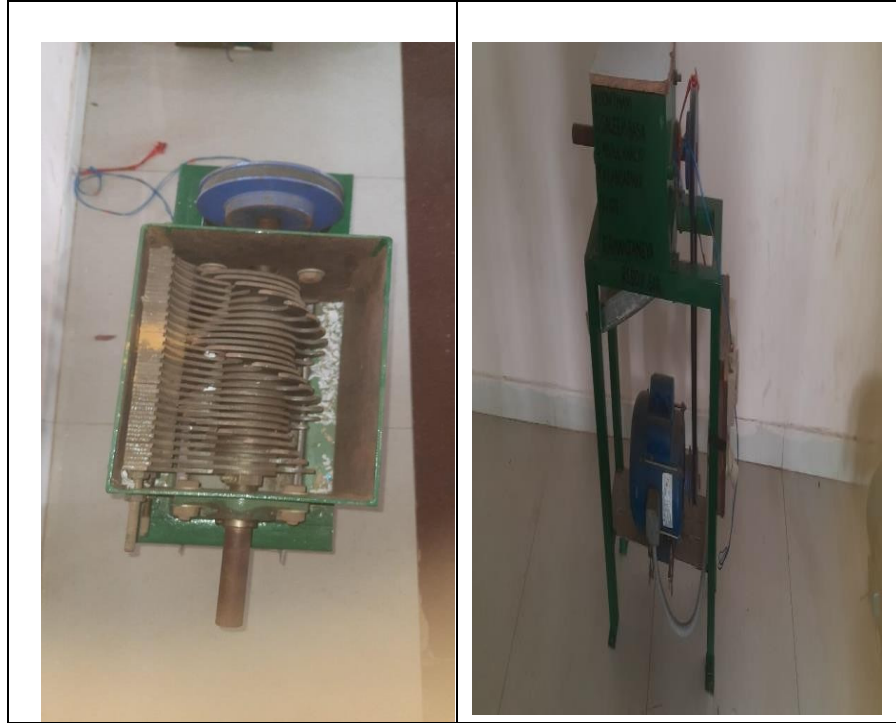
Figure 2: Sectional Views of Single-Shaft Shredder Machine
