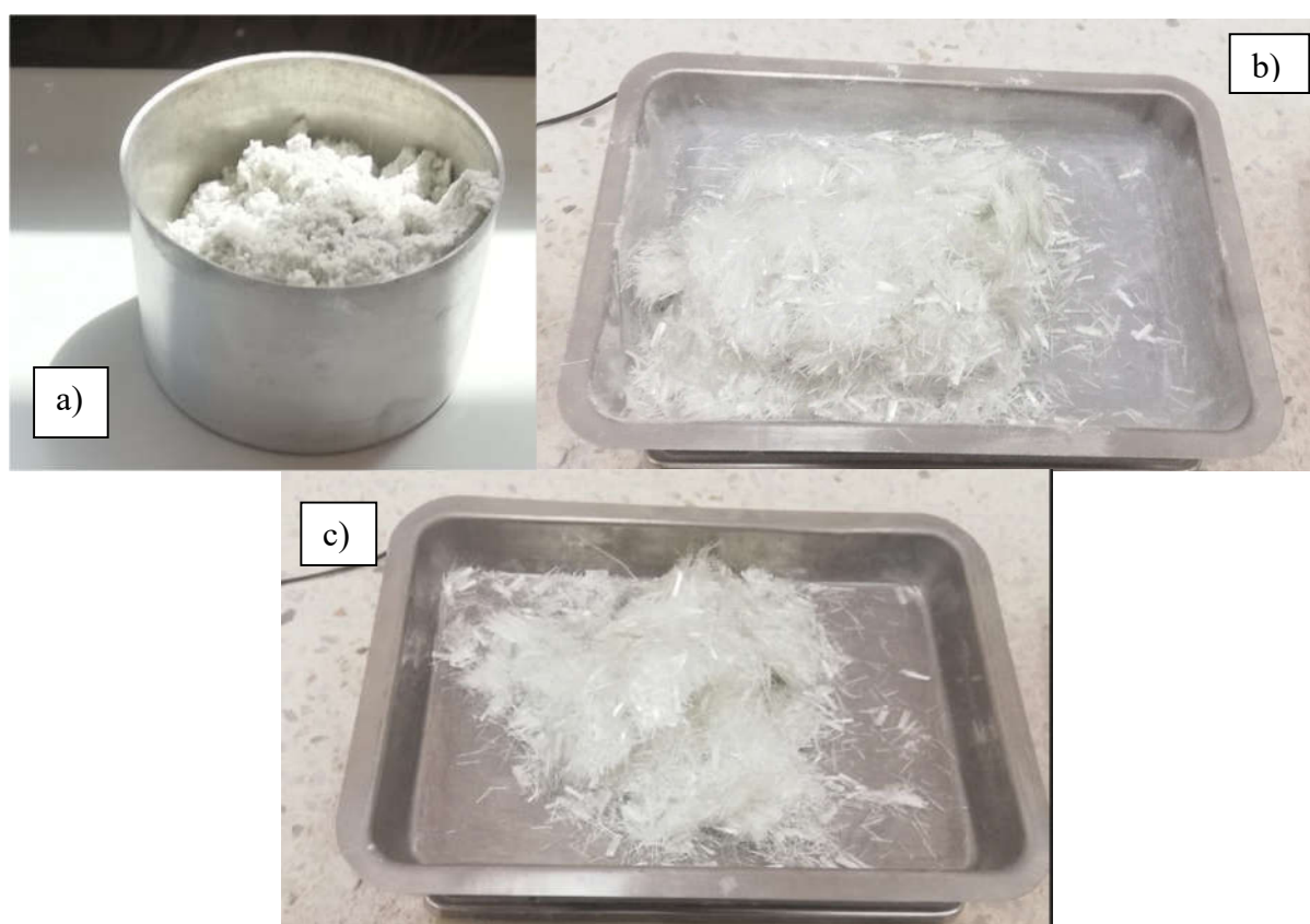
Figure 1. Images of fiber glass materials a) powder b) 6 mm c) 12 mm fiber
